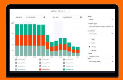
SimbleSense revealed previously unknown inefficiencies, enabling over 50% savings in a single water pump. The platform uncovered a flat energy profile in water pumps as load was changed in the system.
